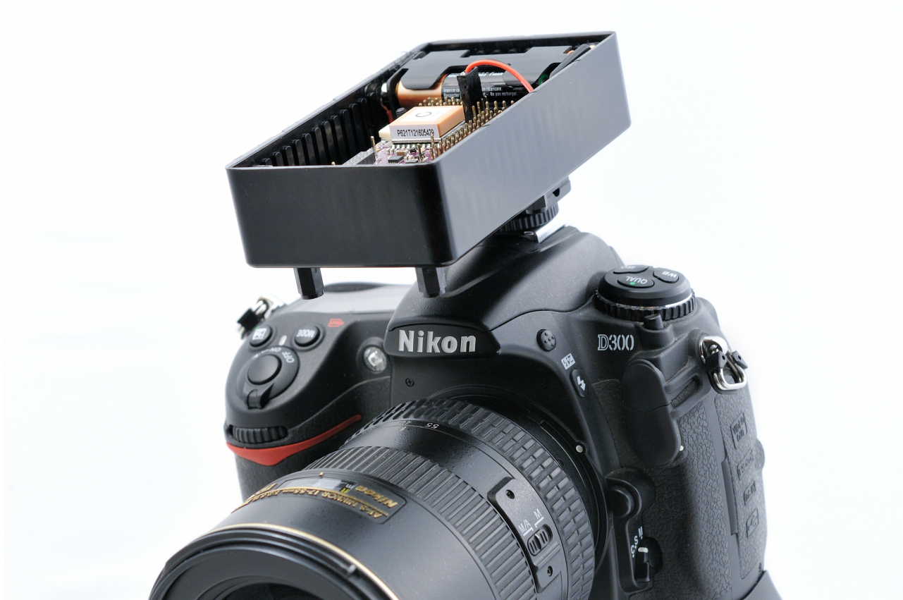
Figure 1: The first prototype of a hot/shoe-mounted case which holds the integrated POS solution.
