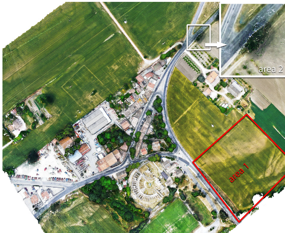
Fig. 4. The Ricina orthophoto calculated out of 27 oblique images and enhanced for crop mark display. The area indicated in red is a down sloping zone which was previously impossible to accurately georeference due to the lack of GCPs and a detailed elevation model. (For interpretation of the references to colour in this figure legend, the reader is referred to the web version of this article.)
