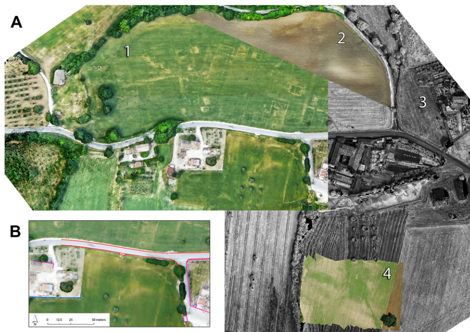
Fig. 6. (A) Integration of several orthophotos, showing crop marks (1) and soil marks (2) in the visible domain, the NIR terrain reflectance (3) and the orthorectification of an image (4) without any useable GCP; (B) shows the comparison between the generated orthophoto and total station measurements of the road and other building structures.
