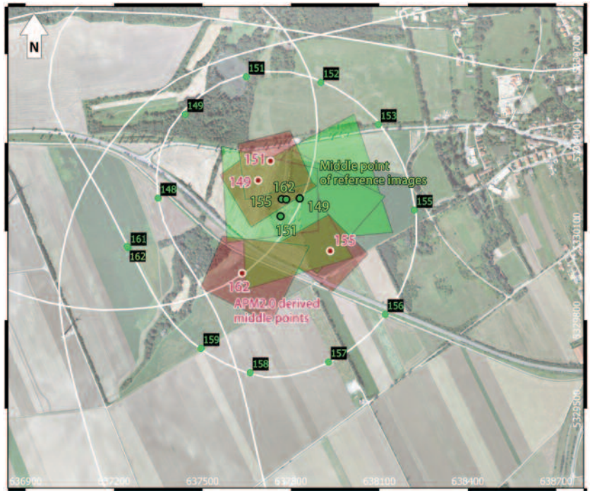
Figure 8. The projected coordinates of the principal image point (middle point) and the footprints of four reference aerial images (green) compared to the results of the APM 2.0. Instead of the GNSS data recorded by the APM 2.0 the additional GNSS receiver was used (red). The flight track (white) of the additional GNSS receiver has an accuracy of a few meters in respect to the reference image location. (illustration by M. Wieser and G. Verhoeven).
