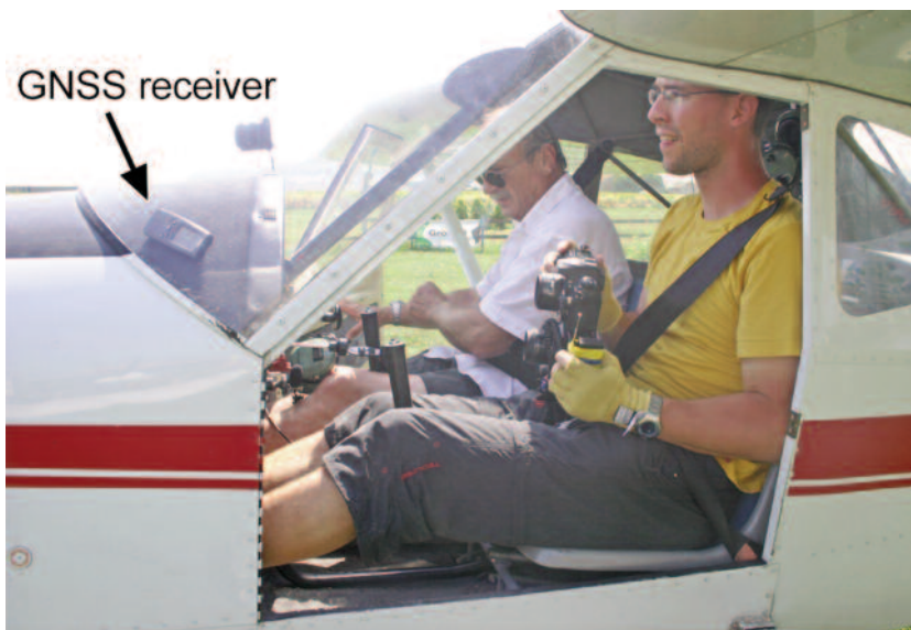
Figure 1. The aerial photographer inside a Cessna 172 holding a two-camera rig while the GNSS receiver is located in the front of the cockpit (photograph by F. Vermeulen).
